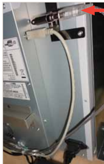
P.7 P.7 USB Extension AM / AF From Dongle to PC. (180 cm - Inch 70,87)
