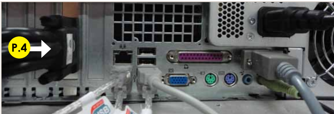
P.4 VGA Cable 4 to Monitors
