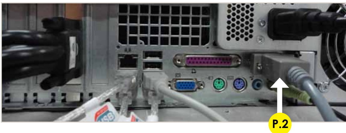
P.2 Serial Cable From PC to Control Board . STRIP (200 cm - Inch 78,74)
